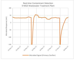
Figure 3 — Real-time microbial signal response to bronopol (microbial biocide) contamination from adjacent airport sewer discharge. Contaminant response demonstrated by negative spikes in the microbial signal.
