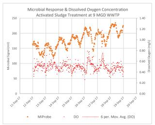
Figure 2 — Microbial response to dissolved oxygen concentration in an activated sludge reaction cell. A moving average of DO was required to reduce noise for visual comparison.
